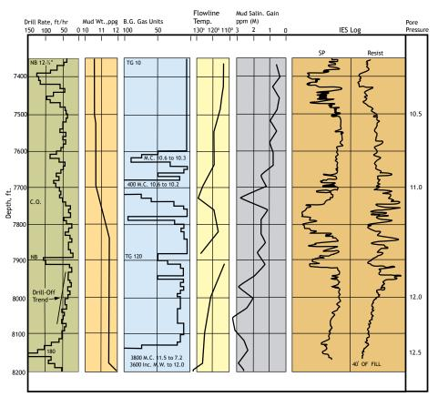
Figure 4.11. Abnormally pressured formations can be identified by electric logs.
