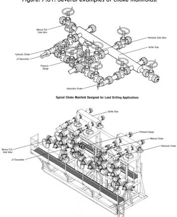
Typical Choke Manifold Designed for Subsea Drilling Applications
