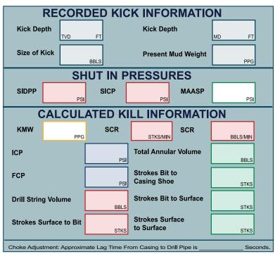
Figure 9.20. D, the pre-recorded section of the kill sheet.
