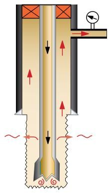
In the case of total lost returns, depending on the severity of the developing underground blowout, pressures may change rapidly.
