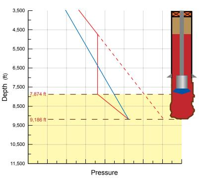
Safe stripping practices involve two primary concerns. There is the mechanical operation itself that consists of the rig-up and operation of equipment, specific assignments for the crew, and careful displacement and volume calculations. Also, since some gas is associated with most formation fluids, consideration must be given to controlling bottomhole pressure in the event of gas migration during the stripping operation.
