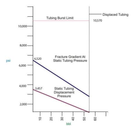
Figure 9.23. A typical bullhead pressure chart.
