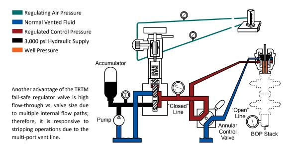
Figure 10.11. Fail-safe regulator valve.
