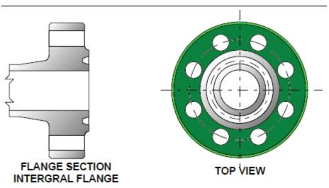
Figure 7.51. An illustration of API Type 6BX Flange.
