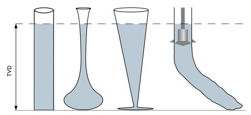
Figure 2.1. Hydrostatic pressure varies with density and TVD.
