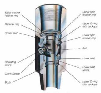
Cutaway view of standard Hydril Kellyguard in open position.
