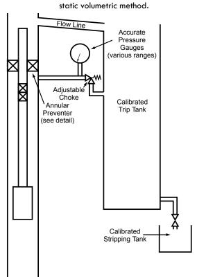
Figure 10.8. Rig layout for combined stripping and static volumetric method.
