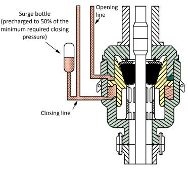
Manufacturer's tables are available for various make and model preventers and should be used as guides for establishing the initial closing pressure.
