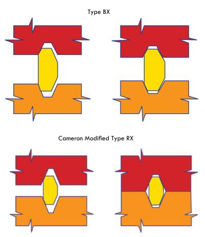
Figure 7.54. Ring joint gaskets.
