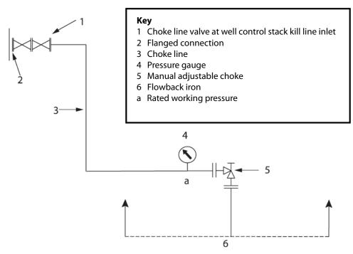
Figure 7.59. A single manual adjustable choke.
