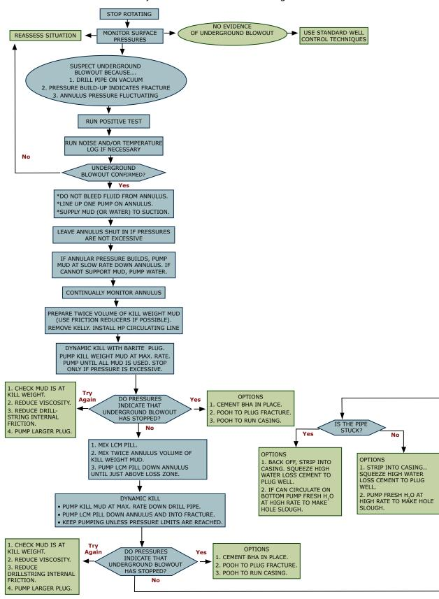
Figure 10.5. Kick off bottom (drill pipe in stack)
