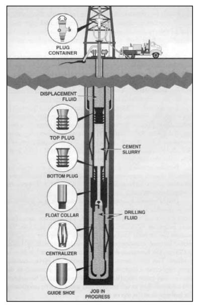
Figure 4.9. Illustration of cementing operation.
