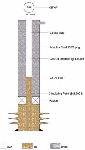
Figure 2.7. Example of a production well.
