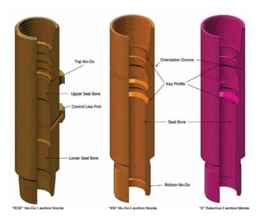
Figure 7.3. Typical wireless landing nipples.
