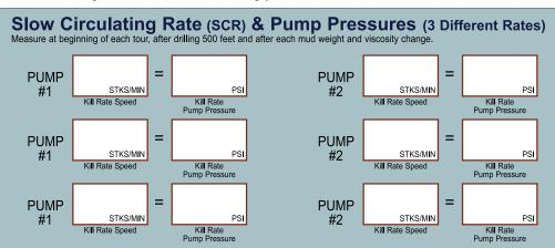
Figure 9.16. C, slow circulating pressure calculations in the kill sheet.
