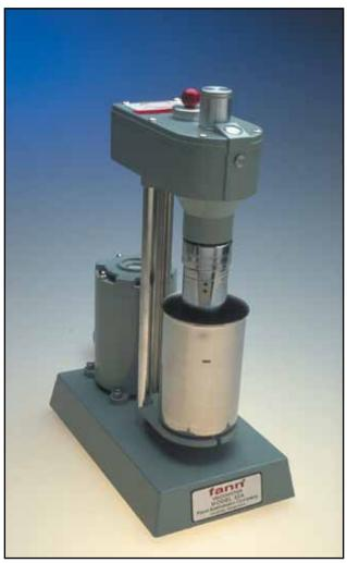
Figure 6.6. Rotational viscometer for measuring viscosity and gel strength.
