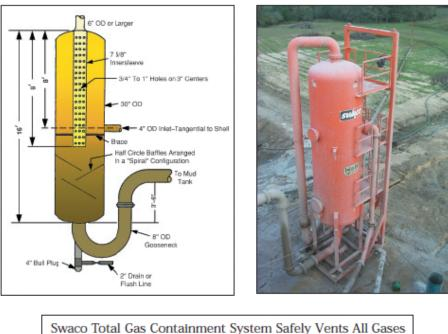
Figure 7.68. Illustrations of mud-gas separators.
