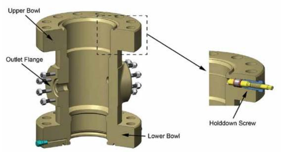
Figure 7.21. A tubing hanger spool.
