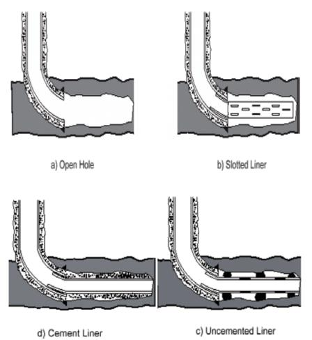
Figure 1.3a. Horizontal well completions types.
