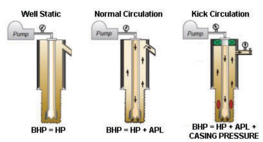
Figure 2.14. Bottomhole pressure varies during different operations.
