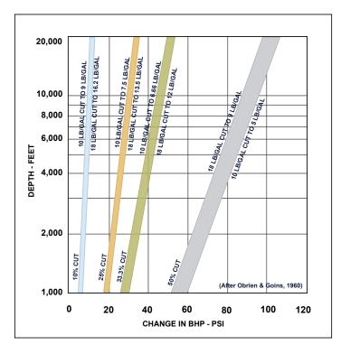
Figure 4.18. Gas-cut mud usually does not cause a reduction in BHP.
