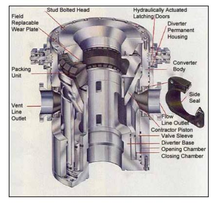
Figure 7.28. An illustration of a diverter.
