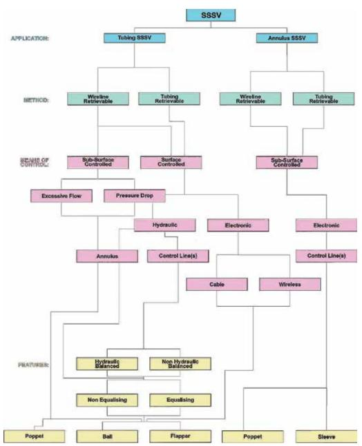
Figure 7.14. A diagram of subsurface safety valve applications.
