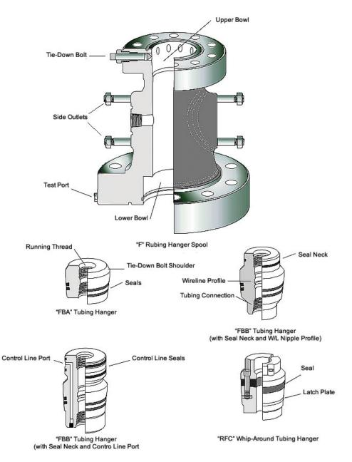
Figure 7.19. Cameron 'F' tubing head and hangers.
