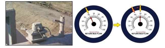
Figure 4.20. Left, a flow rate sensor. Right, an influx of formation fluid will cause an increase in flow from the well.
