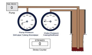
Figure 9.11. Killing a well using the wait-and-weight method.
