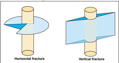
Figure 1.8. Most induced fracture planes are vertical, however shallow formations may exhibit horizontal fractures.
