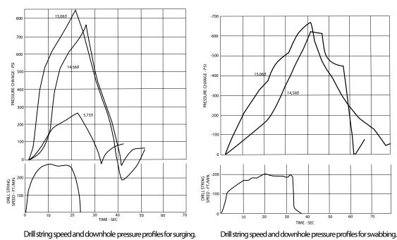
Figure 10.21. 14.2 ppg water-based mud, 5-inch casing based on 90 ft. of pipe movement.
