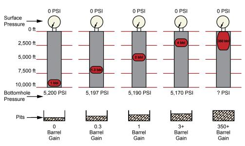
Figure 5.2. Uncontrolled gas expansion.
