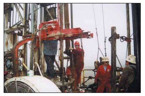
Figure 4.23. Casing operations.
