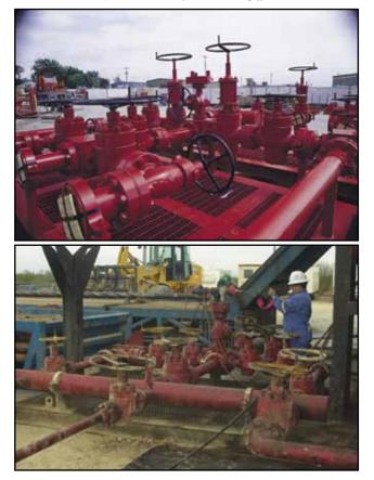
Figure. 7.61. Several examples of choke manifolds.
