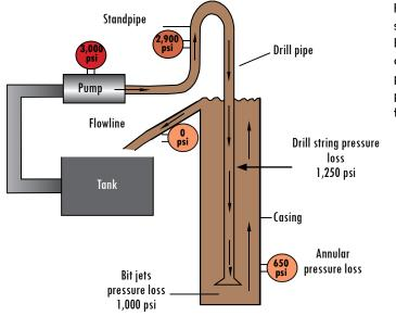
Figure 2.11. Circulating pressure.
