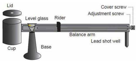
Figure 6.3. Details of a mud balance.
