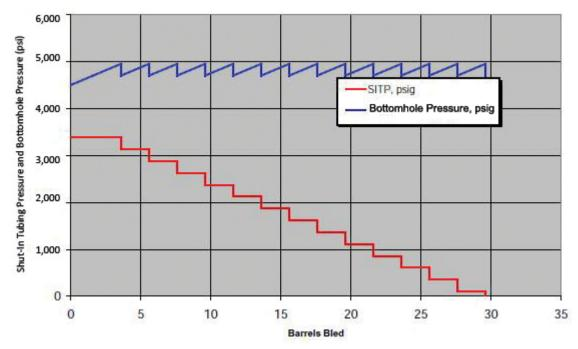
The example worksheet uses a safety margin of 200 psi and a working margin of 252 psi. Margins this large are possible only with relatively strong reservoir fracture pressures (formation integrity). Often, safety margins must be only 50 to 100 psi and working margins 100 psi or less.
