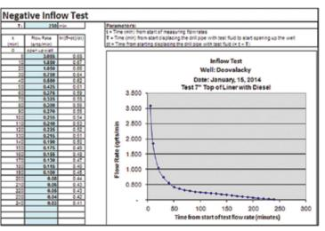
Figure 3.11. Negative inflow test showing passing results.
