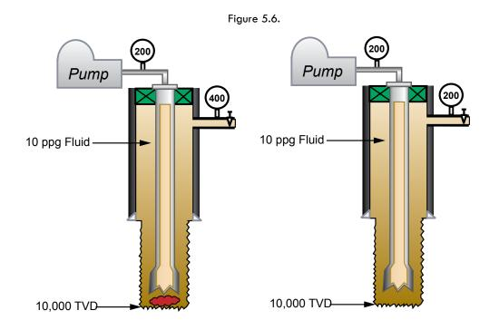
Well data: 15 bbl pit gain SIDPP 200 psi SICP 400 psi CMW 10.0 ppg Annular capacity at BHA is 0.029 bbl/ft Assume that the influx in the illustrated well is near the bottom of the well. 1. Estimate the height of the influx.
