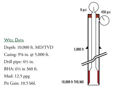
The annulus around the BHA represents the highest pressure per barrel  $(0.65 \div 0.02908 = 22.35 \text{ psi/bbl})$  and therefore provides the greatest safety, however the BHA is only 360 feet long and in this case it is probably safe to use the lower value. However, it must be stressed that this is a well-specific judgment. Other factors, such as formation strength must be considered when selecting pressures and bleed-off cycles.
