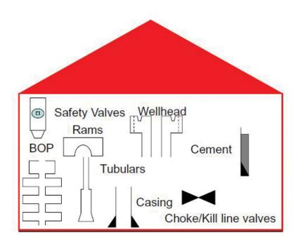
Figure 3.2. An example of elements that form the barrier envelope.
