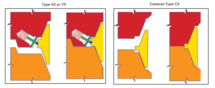
Figure 7.55. Ring joint gaskets.
