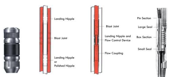
Figure 1.15. Left to right, a bridge plug, placement of blast joint, flow collar placement, safety joint.
