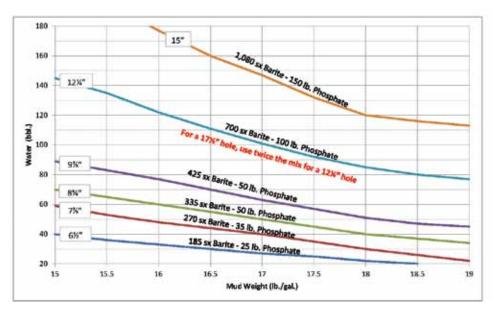
Figure 4.3. Barite plug mixtures for 300 feet.
