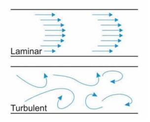
Figure 6.4. Laminar and turbulent flow.
