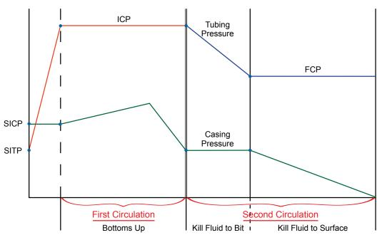
Figure 9.10. The driller's method.
