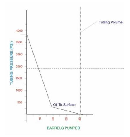
The slightly higher hydrostatic head on the formation is maintained during the kill operation reducing the chance of influx of the formation fluids. As the kill fluid moves up the tubing, the back-pressure held on the tubing head is reduced. This can be shown in the form of a graph with tubing head pressure against time (assuming a constant pumping rate) or tubing head pressure against quantity pumped (refer to figure 9.21).
