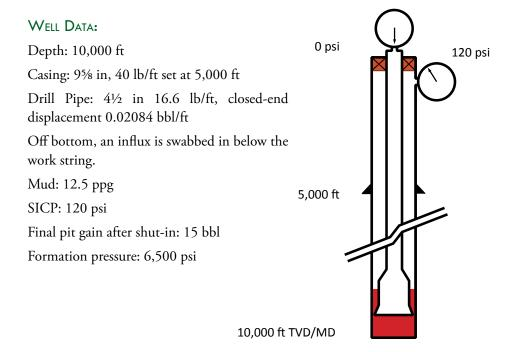
The closed-in displacement of the  $4\frac{1}{2}$ -inch drill pipe with tool joints is 0.02084 bbl/ft, therefore each 93 feet stand displaces 1.94 barrels (0.02084 \* 93 = 1.94). After the proper equipment is rigged up, a detailed safety meeting is held. During this meeting the crew is informed as to the details of the operation and individual tasks are assigned and explained.
