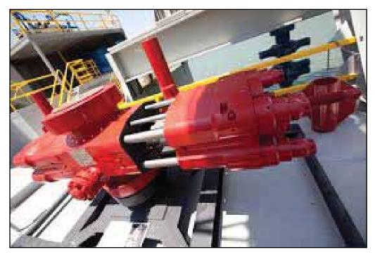
Figure 7.46. An example of drilling spools.
