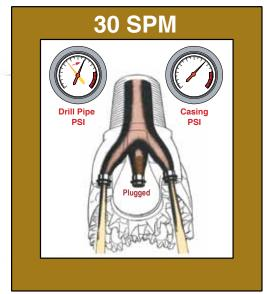
If the all the bit jets are obstructed and the amount of pressure increase cannot be tolerated at kill rate speed, the bit jets can be cleared by using wireline to blow out the bit jets or perforate the drill pipe above the bit. The casing pressure must be controlled while waiting on a wireline unit to perforate the drill pipe or blow out the bit jets.
