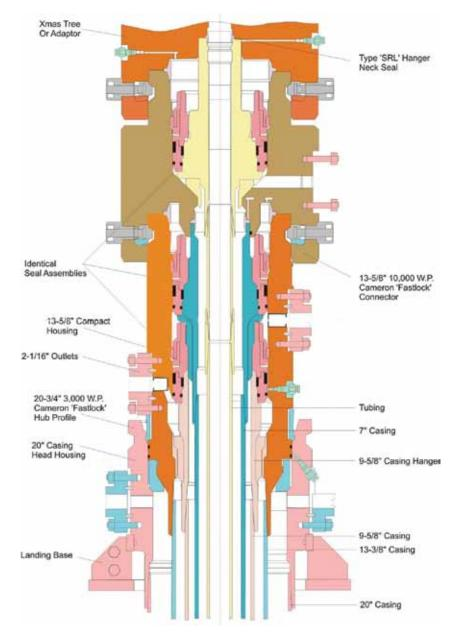
Figure 7.22 An illustration of a typical compact wellhead.
