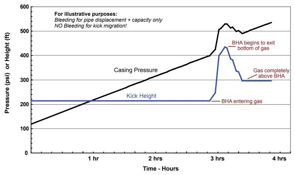
Figure 10.17 was developed using 1.94 bbl/stand as calculated. It is interesting to note that if the closed-in displacement were rounded up to two bbl/stand — a seemingly small adjustment — the well would be underbalanced by 150 psi by the time the bit was at bottom.
