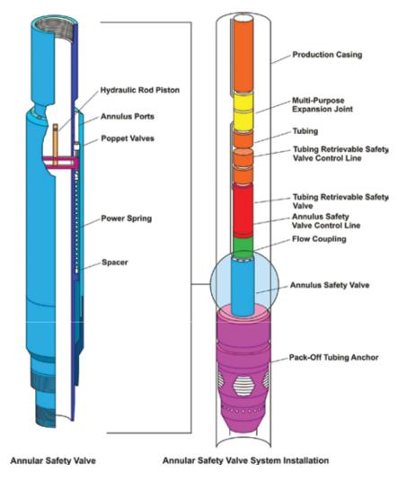
Figure 7.18. A typical annular safety valve system.
