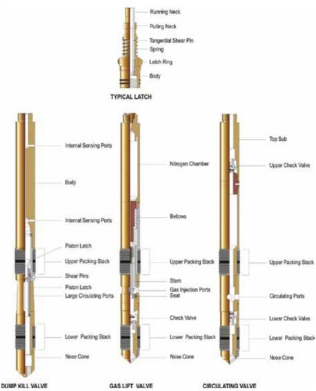
Figure 7.13. Types of SPM valves.
