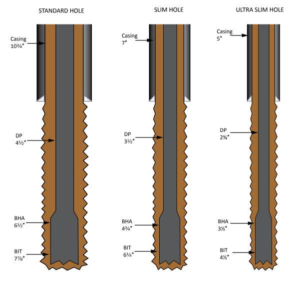
Figure 10.18. Difference in well geometry.
