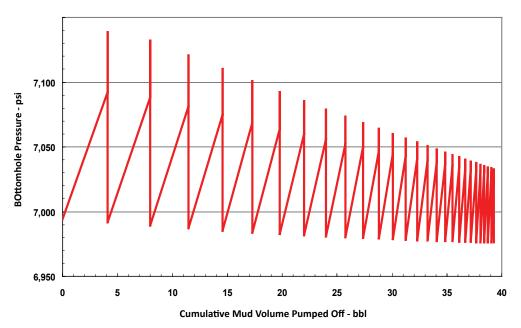
Figure 9.44. Lubricate-and-bleed.
