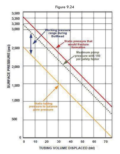
The velocity of the gas/kill fluid interface should be 1,000 ft per hour divided by 60 minutes/hour. Velocity = 1,000 ft per hour  $\div$  60 minutes/hour = 16.7 ft per minute. The capacity of the tubing is calculated: Tubing Capacity = ID<sup>2</sup>  $\div$  1,029.4
