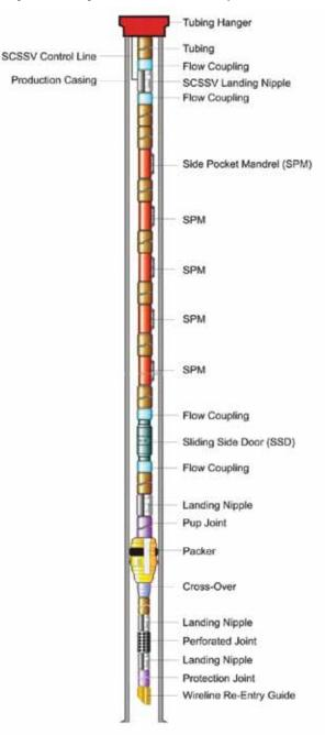
Figure 7.1. A generic well oil well completion.
