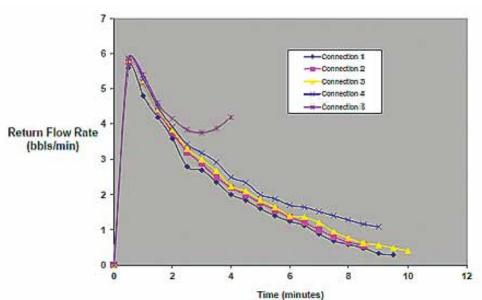
Figure 4.21. "Finger printing" return rate during connections.
